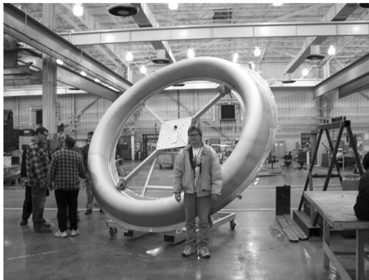
Fig. 6 A fully SPF formed 5083-SP jet engine leading edge nacelle Inlet made by FSW butt welding of four separate segmented blanks prior to forming
